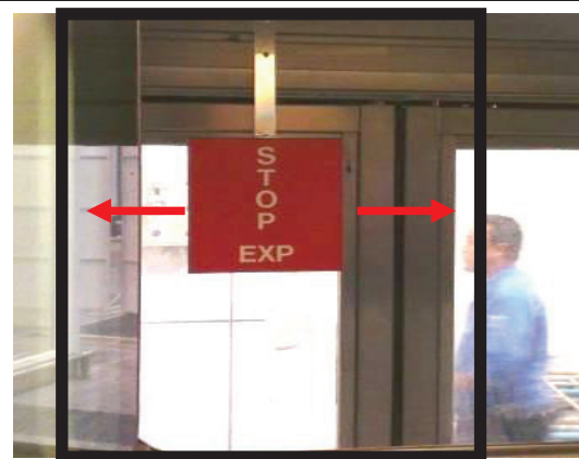
Pic 2- Stop marker shall be within the square cab window
