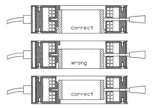
The Bearing inner ring stops inside the induction coil are for positioning at the right depth. To have an equal heating in the bearing inner ring, the position of the bearing inner ring must always be in the middle of the induction coil as shown on the drawings above.
