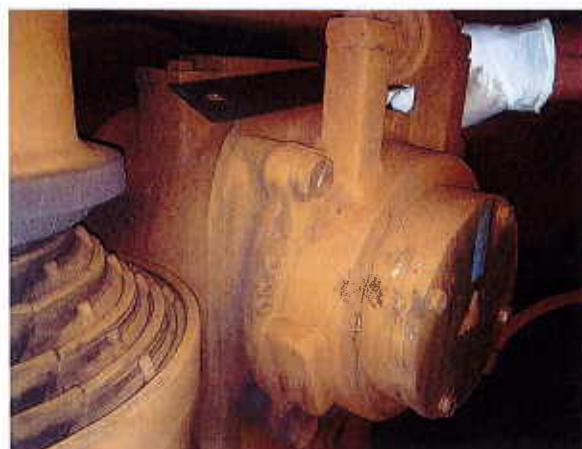
Figure 15 - Adding or removing shim accordingly
