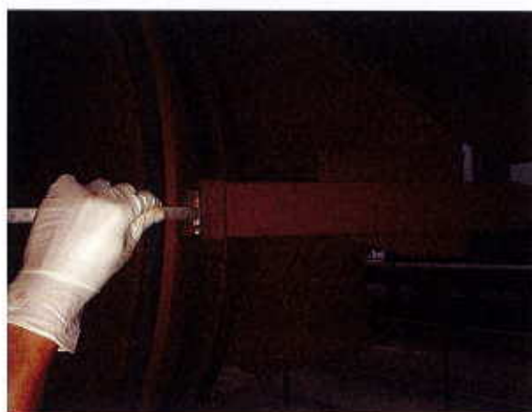
Figure 13 - Measuring the clearance of KELSAN Wheel Flange Lubricators
