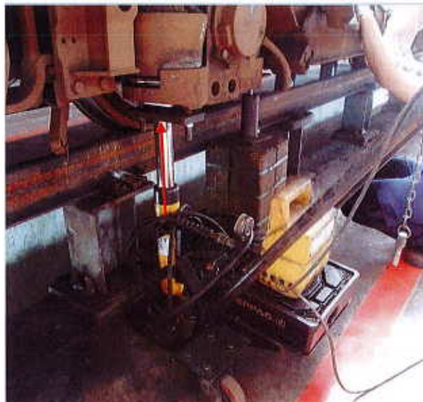
Figure 16 - Lift up the primary spring using hydraulic jack (1)
