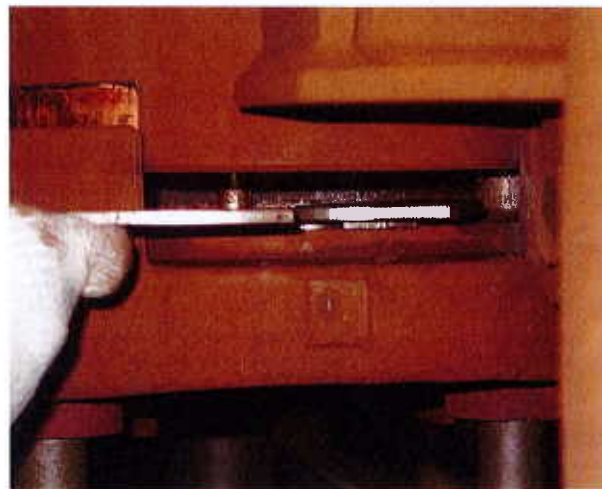
Figure 19 - Remove or add on shimming on the primary spring
