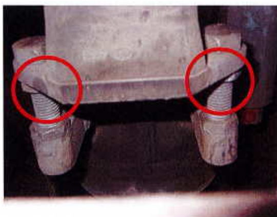
Figure 27 - Screw/bolt to adjust the Z9
