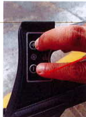
Figure 11 - Vacuum function side button B1 (+/-)
