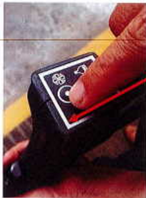
Figure 10 - Speed button B3 to activate vacuum function
